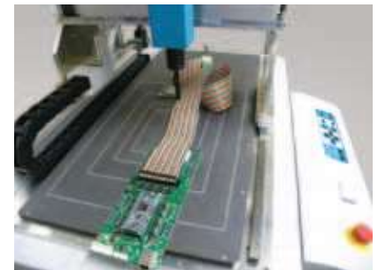
Long items can be scanned while they protrude from the device.
