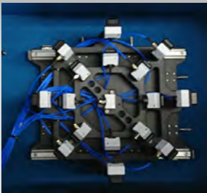
Customization example Beam test jig
